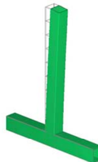
(b) Displacement of complete destruction (10 mm).
