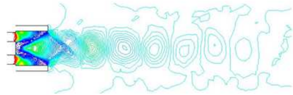
Figure 2-10. Areas of compressions and expansions in outlet of overcritical air flow.
