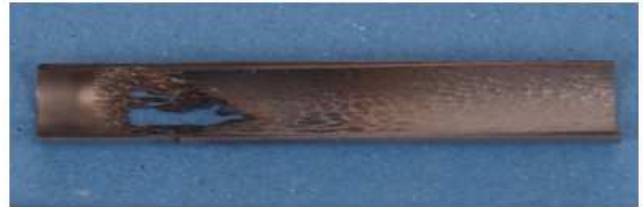
Figure 3-11. Erosion of the mixing tube wall
