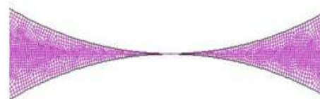
Figure 2-1. Mesh between drums (cutout of the whole model).
