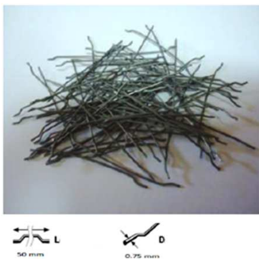
Figure 1: « HE++ 75/50 » Steel Fibers.
