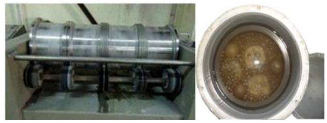
Figure 5: Abrasion testing machine.
