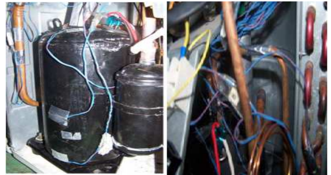
Figure 3. Compressor with thermocouples.
