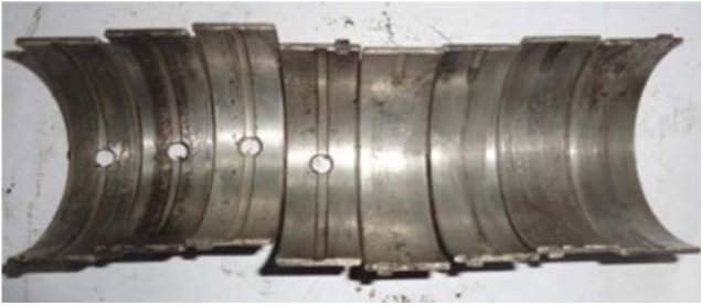
Figure 3. Damaged Crankshaft Bearing.
