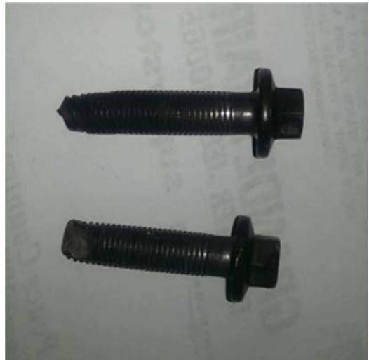
Figure 5. Damaged Connecting rod bolts.
