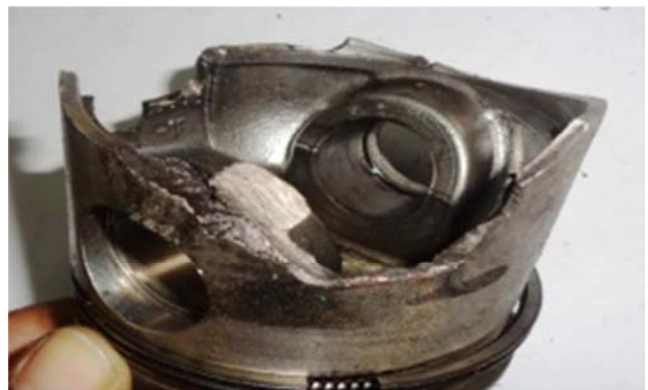
Figure 8. Cracked Piston.
