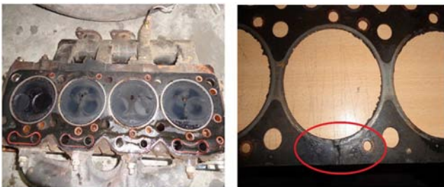
Figure 9. Cylinder head & Head gasket.
