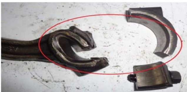
Figure 7. Bent Connecting rod.
