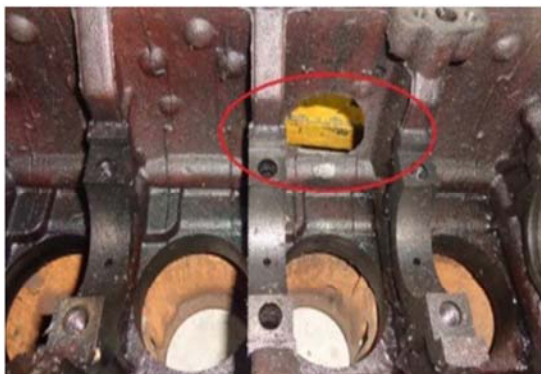
Figure 6. Cracked engine block and crankshaft.
