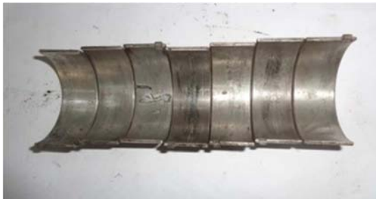
Figure 4. Damaged Connecting rod bearing.
