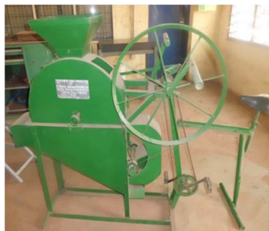
Figure 1. Pictorial view of the groundnut decortivating machine.
