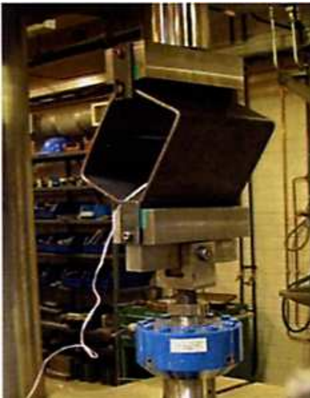
Figure 1. Distortion testing of CFRHS.
