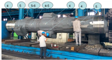
Figure 8. ASTM level and ultrasonic test for CAP1400 main pipe hot section hollow forgings.
