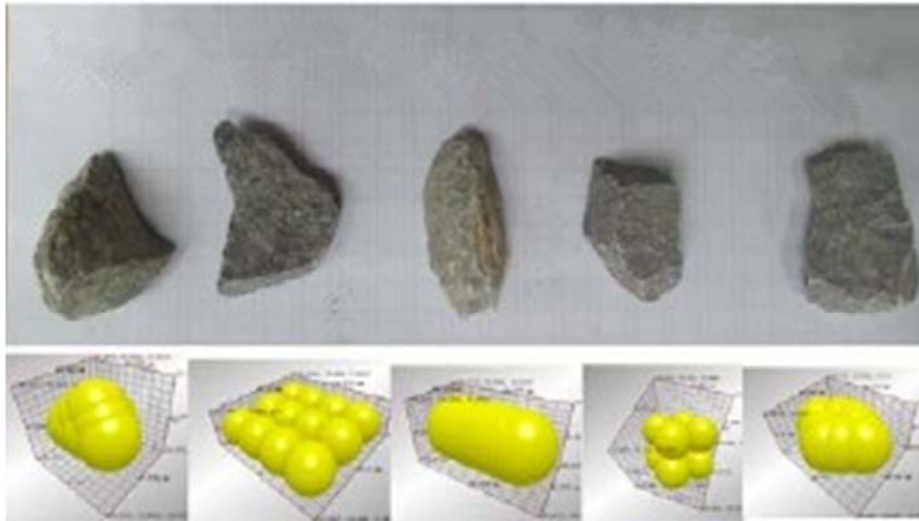
(a) Five kinds of granulated particles
