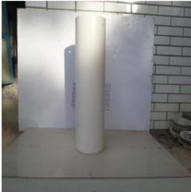
(b) bottomless cylinder experiment device
