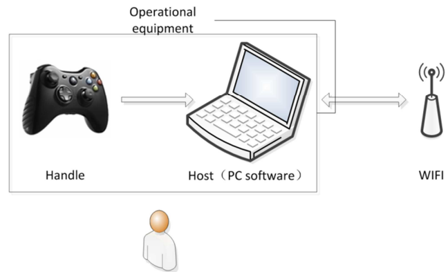
Figure 5. Ground Control Terminal Architecture.
