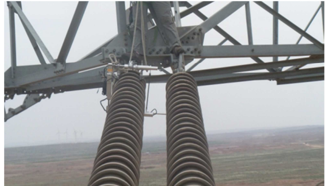
Figure 8. Insulator Inspection Robot Field Test (+800kV).
