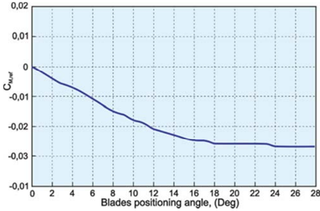
Figure 6. Moment coefficient C_{M,ref} depending on the angle of attack for the NACA 0016 profile.
