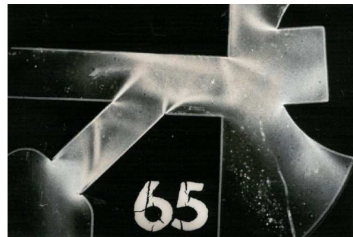
Figure 2.3-1. Schlieren photograph of shock waves in the overcritical flow
